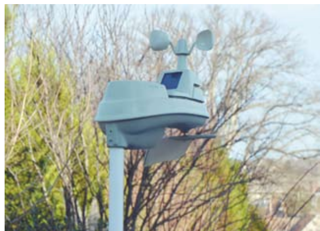
This Acu-rite Personal Weather Station transmits precipitation, wind speed and direction, humidity and other meteorological data through a wireless connection.
